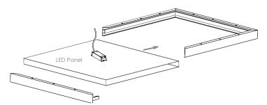
(5) Take out one frame, connect the panel light to driver, insert the panel light into the frame.
