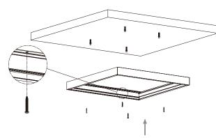
(4) Knock the plastic anchor into ceiling, fix the Aluminum frame on the ceiling by screws.
